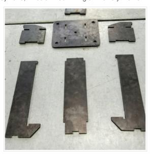
When the parts where retrieved, I started cleaning off the burrs and fitting it together like a jigsaw puzzle.
