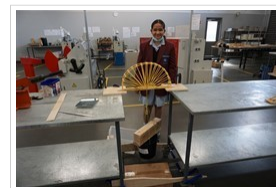
ENS09C Indira D'Sylva 2nd place (Bridge 431 grams, failed at 13kg)
