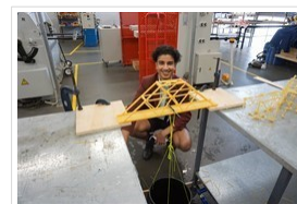
ENS09D Eishman Brar 2nd place (Bridge 300 grams, failed at 11.2kg)
