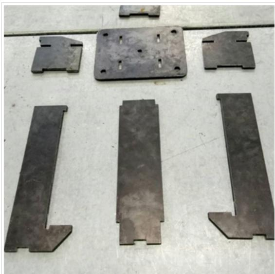
When the parts were retrieved, I started cleaning off the burrs and fitting it together like a jigsaw puzzle.
